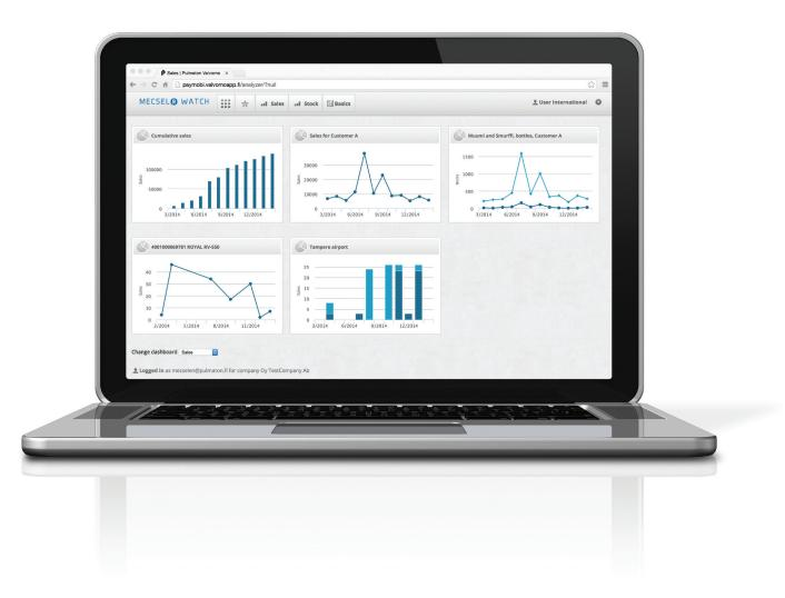
Mecsel Smart plugs into the vending machine's DEX port on MDB or to MDB peripheral on EXE configuration. The telemeter reads the DEX file and transmits it to a handheld device or to a remote server. The data is organised, stored and processed by Mecsel® Watch. The software application then creates reports as required. These reports can be exported to feed into operators own enterprise business application.
